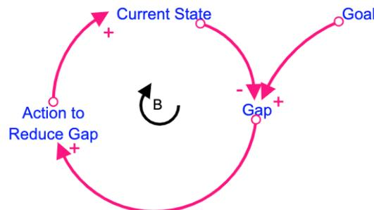
In our homes, thermostats operate on this concept, measuring the actual temperature in a room and comparing it to a goal temperature. If the actual temperature is too low, the heat turns on in an effort to reduce the gap; if it is too high, the heat turns off, allowing the room to cool. This process repeats indefinitely, causing the heater to turn on and off at just the right times to maintain the desired temperature.
