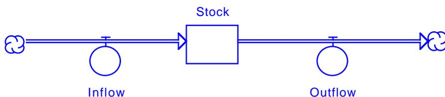
**map** — a pictorial representation of a system, usually with a causal loop or stock-flow diagram.
