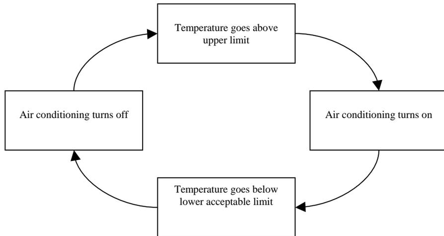
Figure 3-4. Household thermostat as an example of a negative (balancing) feedback loop
